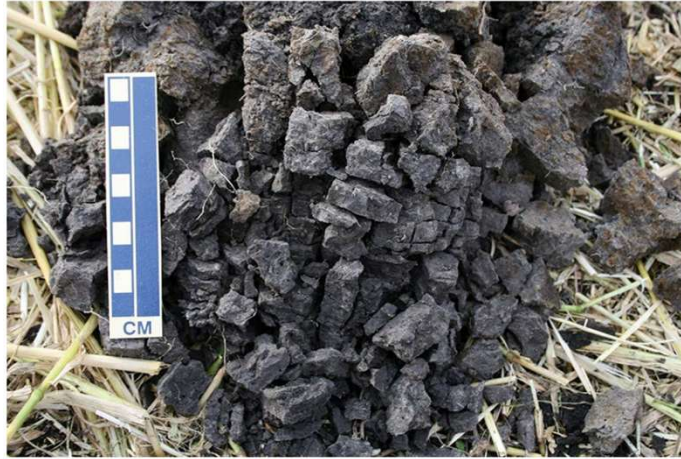
Figure 3: Peds with angular blocky structure.
