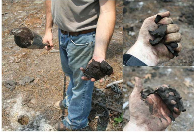
Figure 13: A field test on a soil with a moderately fluid manner of failure class.
