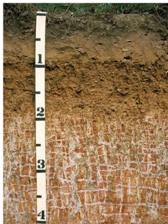
Figure 9: A soil in which a reticulately mottled zone with plinthite (darkest red colors) is below a depth of about 2 feet.
