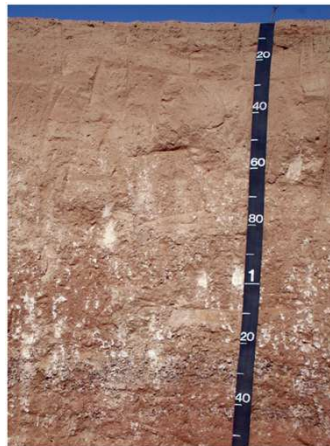
Figure 8: Masses of secondary calcium carbonate (white bodies below a depth of about 60 cm) in the calcic horizon of an Aridisol.
