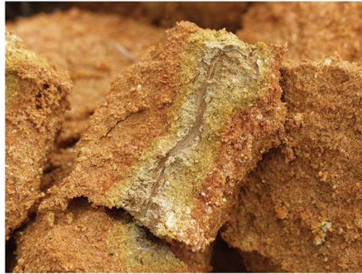
Figure 12: Redoximorphic features that consist of a redox concentration, as an iron mass (reddish area along ped surface) and an iron depletion (light-colored area surrounding the root channel in ped interior).
